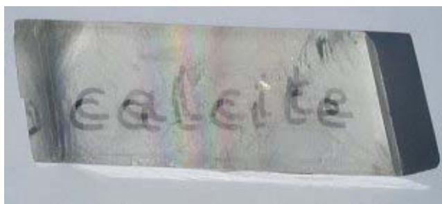
Figure 57.1: Birefringence in a sample of Iceland spar. (Credit: Jo Edkins, http://gwydir.demon.co.uk/jo/minerals/index.htm )
